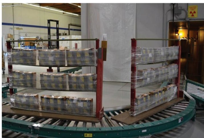
Blueberries ready to enter the x-ray unit at the irradiation facility (Credit: Anuradha Prakash)
