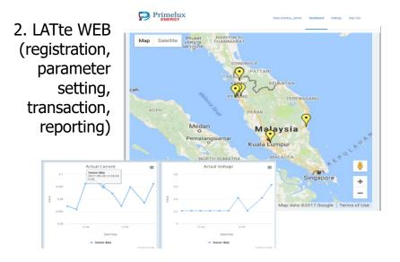
Once failure light detected, the device automatically triggers the Maintenance Team via Smart Phone to repair or replace malfunctioned light.
