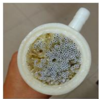
Activated Carbon Grafted Hollow Fiber, Composition: 15% PES+ 0.3% Activated Carbon in NMP
