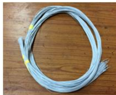
Activated Carbon Grafted Hollow Fiber, Composition: 15% PES+ 0.3% Activated Carbon in NMP
