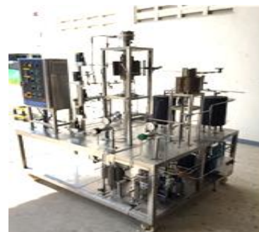
Autothermal reforming reactor for bio-methanol production ( 0.025 L/day)
