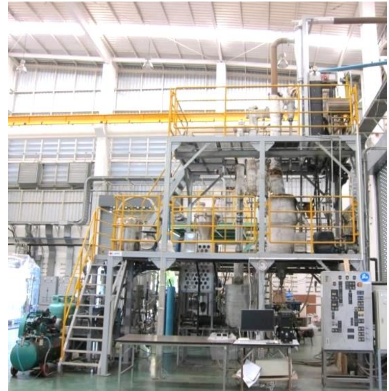
Circulating Fluidized Bed Pyrolyzer 0.2 Ton Biomass/Day
