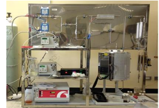
Syngas production by steam reforming process
