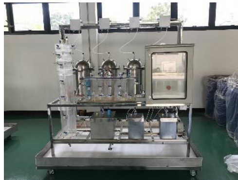
SLBR-UASB (Sequential leach bed reactor with upflow anaerobic sludge blanket) (2-stage digestion) 30 L/day
