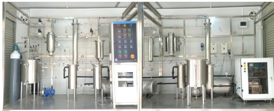
Bio-methanol production from biogas (Semi-pilot scale : 1 L/day)
