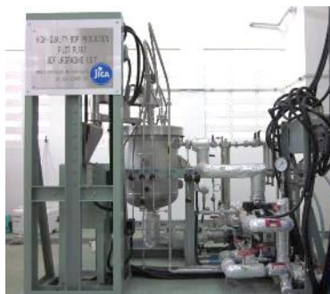
Biodiesel upgrading unit (H-FAME, 100 L/batch)
