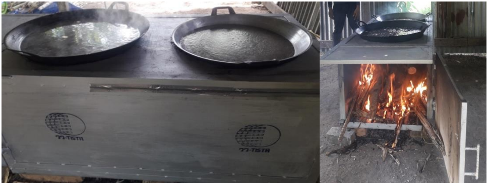
Biomass stove type 3 used wood fuel about 50 kg /40 liters sugar can juice
