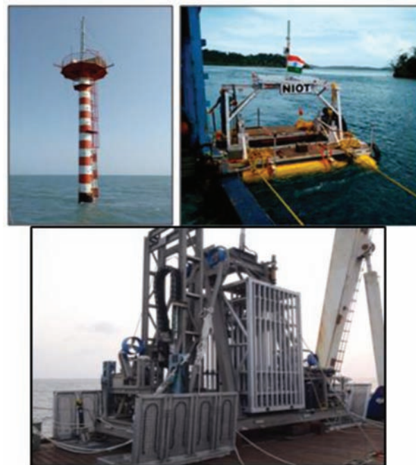
Figure 2: (a) Offshore wind assessment station, (b) Marine current turbine, (c) Autonomous coring system
