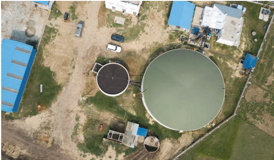
Figure 1: Gandaki Urja Pvt. Ltd., Kotre, Pokhara (Waste processing capacity: 45 tons/day; Gas Output: 4000 m 3 biogas /day; End Use: Bottling and sale (>200 cylinder/day); Organic Manure production: 15 tons/day)
