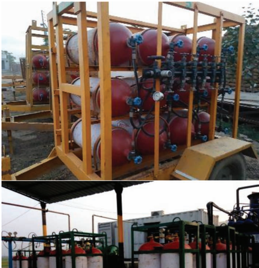
Figure 3: Compressed natural gas cylinders in case
