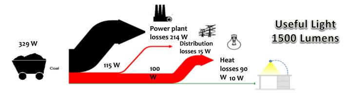
**One improvement:** 329 W to 83 W: 75% less energy by switching from incandescent to Compact Fluorescent Lamps (CFL) – improving end use technology (Factor 4).
