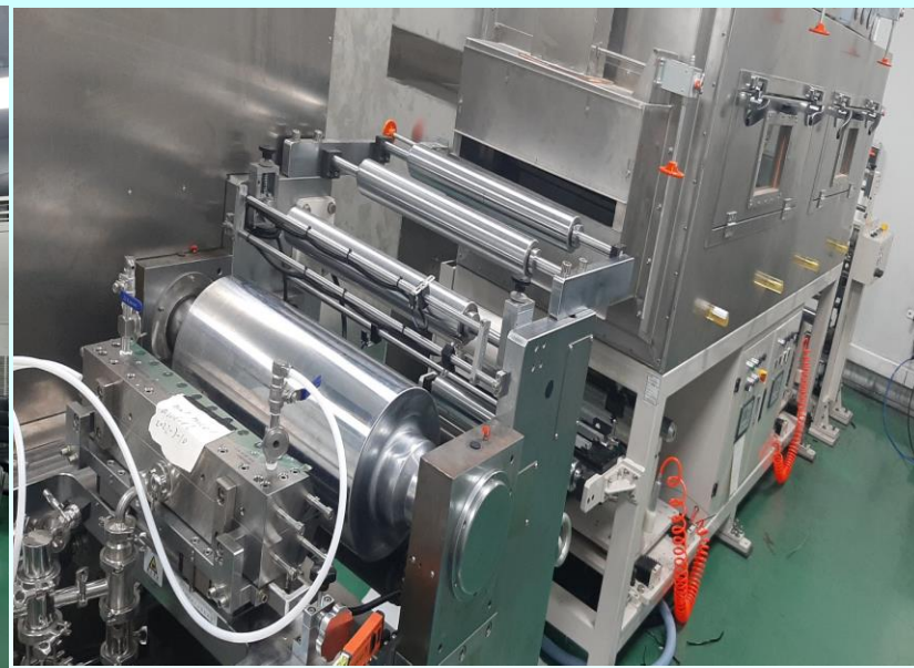
Assembly Line inside 1% RH Dry Room
