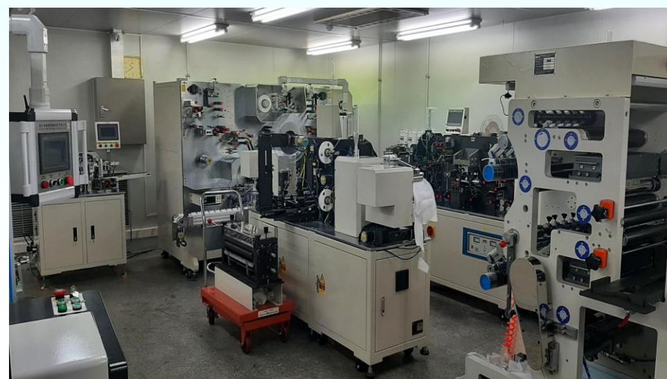
Assembly Line inside 1% RH Dry Room
