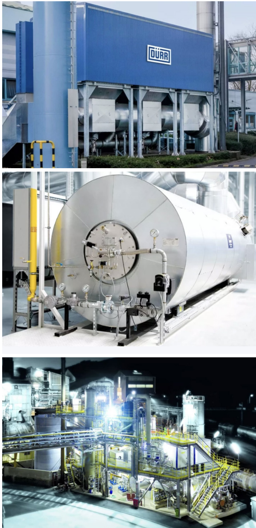
Figure 2.15 (Top) Regenerative thermal oxidation, (Middle) Recuperative thermal oxidiser, (Bottom) Thermal incinerator. Source: https://www.durr.com/en/products/environmental-technology/exhaust-gas-and-air-pollution-control/oxi-x-thermal-processes .
