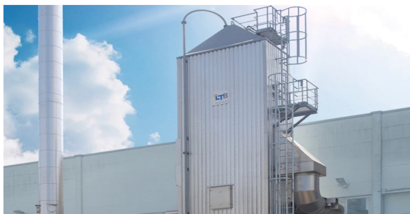
Figure 2.19 Cross-flow packet bed filters. Source: https://www.durr.com/en/products/environmental-technology/exhaust-gas-and-air-pollution-control/sorpt-x-sorptive-processes/sorpt-x-sq .
