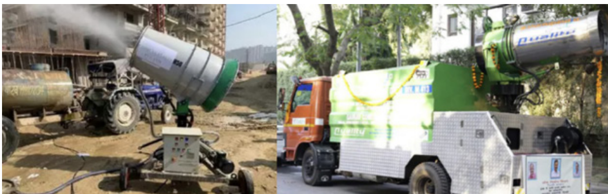
Figure 11: Vehicle mounted mist sprays (Source: Deshpande, 2023)
