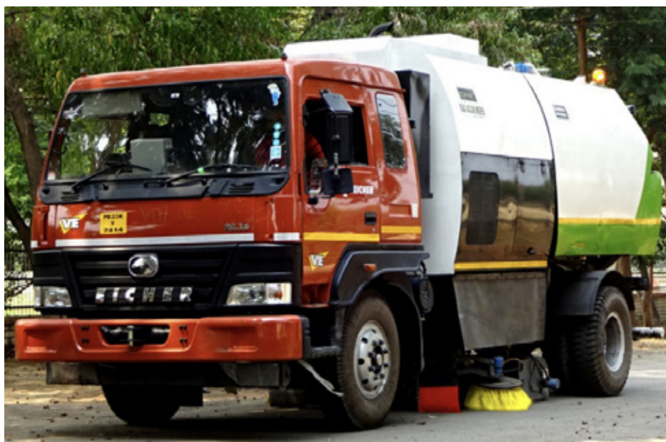
Figure 8: Mechanical Road Sweeping Trucks (Source: Choudhary, 2023)
